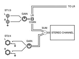
**Dual Stereo Inputs** Each stereo channel has two independent stereo inputs, ST1(3) and ST2(4). For convenience, one uses RCA phono connectors, the other uses TRS jacks. The two inputs mix together to feed the channel strip, or ST1(3) can be routed direct to the LR mix instead, leaving ST2(4) to feed the channel. This provides a very flexible arrangement for mixing up to four stereo sources.
