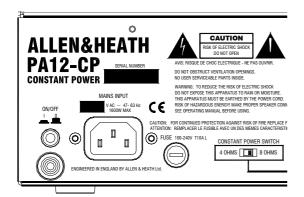
To avoid any unexpected audible clicks or thumps turn connected power amplifiers down or off before switching the console or any other signal equipment on or off. The built-in amplifiers include an automatic turn on delay for this purpose.
