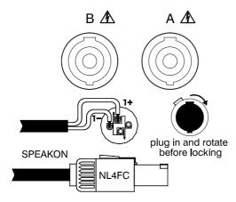
No amplifier output? Check that the Speakon® plugs have been rotated and locked into position.
