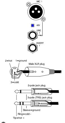
Balanced and unbalanced connections
