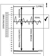
sound peaks. need to consider the matching between the microphones and the (gain), channels inserted equipment (operating level and trims), channels to the mix (faders), and outputs into the amplifiers (level trims). The diagram here illustrates the principles of signal dynamics.
