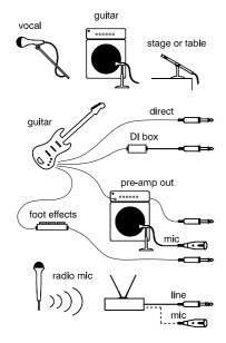
MIC INPUT XLR input for connecting microphone level signals in the range -63 to +5dBu. These are balanced and wired pin 2 hot. Use low impedance microphones (less than 600 ohms) and professional grade mic cables (2 core with shield) for best performance. You can also use these inputs with DI boxes and other low level sources.
