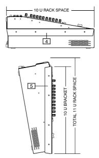
The top panel assembly needs to be removed from the base to gain access to the screws that hold the trims and ears in place. Ensure that you have a suitable work surface with adequate lighting and clear of any objects which may scratch or damage the console panels. Tools required include a number 2 Pozi and T10, T15 and T20 Torx screwdrivers.
